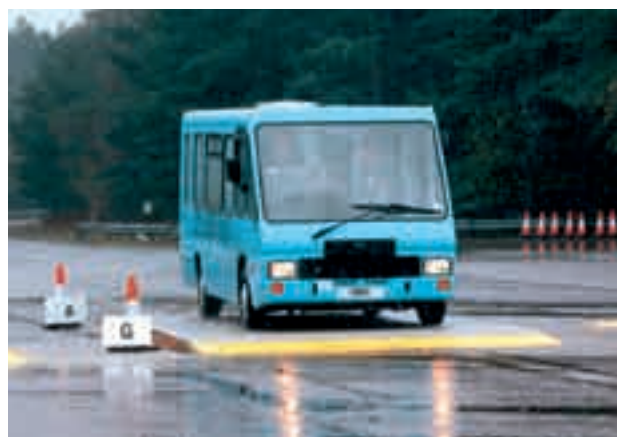
Fig. 2.1 Bus trials over flat-top humps
