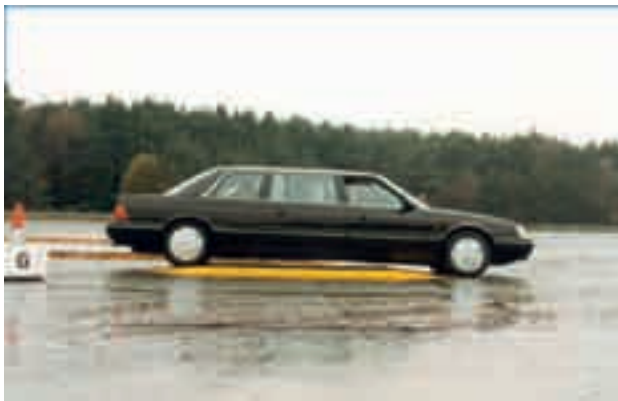
Fig. 4.1 Track trials to examine grounding of vehicles
