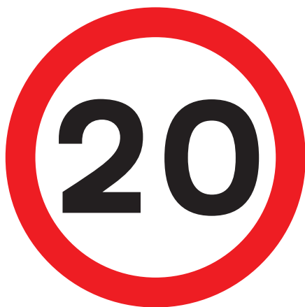
Fig. 3.4 20 mph limit and repeater sign. Diagram 670
