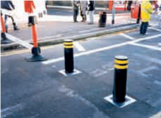
Fig. 3.7 Rising bollards raised and lowered
