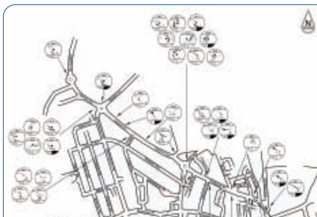
“Bubble diagram” showing locations of collisions as part of a route safety study
