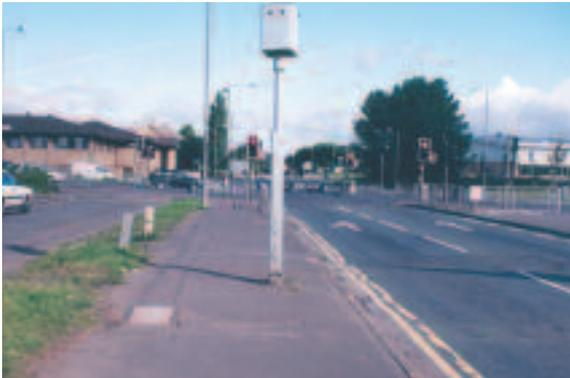
The objective of red light cameras at signal controlled junctions is to reduce the number of accidents caused by drivers' non-compliance with a red signal. Like speed cameras, the equipment automatically gathers photographic evidence of vehicles not complying with the red signal to which it is linked. The evidence needs to be studied by a police officer, and offenders are then issued with a conditional offer of fixed penalty.
