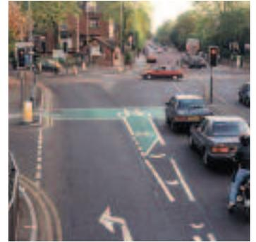
4.20 Problems can arise at uncontrolled junctions if there is any obstruction to drivers visibility. For example, this could be due to the building line, vegetation, parked vehicles or overtaking vehicles being masked by the vehicles being overtaken (despite the Highway Code stating that drivers should not be overtaking in these circumstances).
