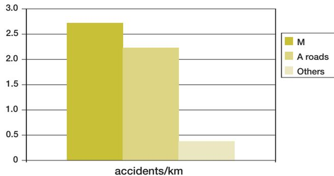
Fig 3.3: Accidents rates (per 108 vehicle-kms) by road class, GB 1999
